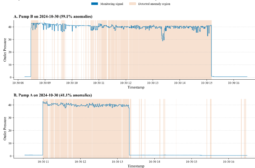
Figure 3. Time-series operating regimes with detected anomalous intervals: (A) Pump B on 30 October 2024; (B) Pump A on 30 October 2024
