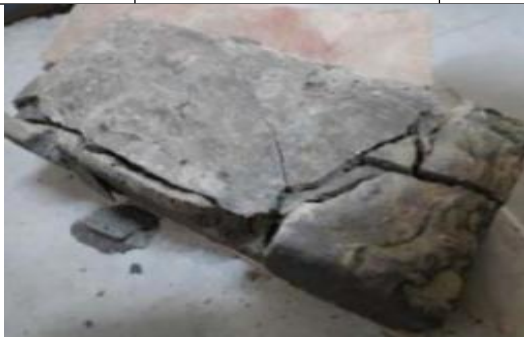
Fig.7 Compressive Strength test on Brick CTM.
