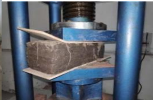
Fig.8 Failure on Brick due to By Compressive load
