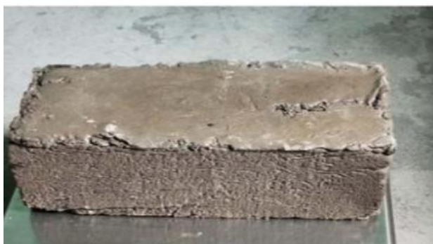
Fig.6 Plastic Sand Brick
