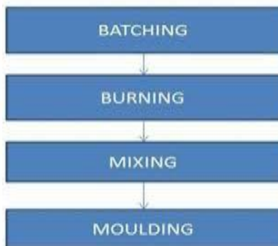
Fig. 2 fabrication process of plastic sand bricks
