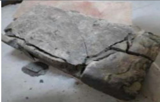
Fig.7 Compressive Strength test on Brick CTM.
