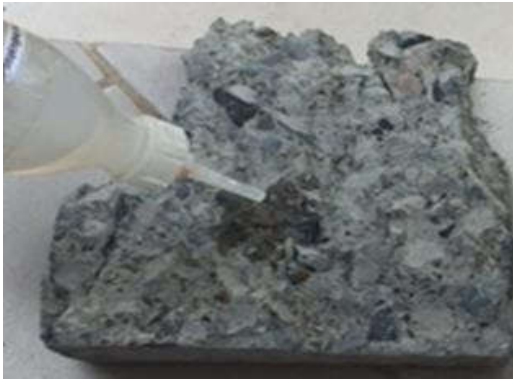
Fig. 11 Corrosion test-normal concrete
