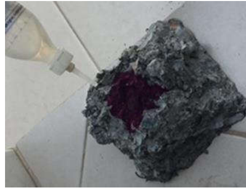
Fig. 12 Corrosion test-concrete with 2% Steel Scrap
