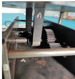
Fig.13- Rack & Pinion arrangement
