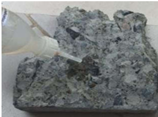
Fig. 11 Corrosion test-normal concrete
