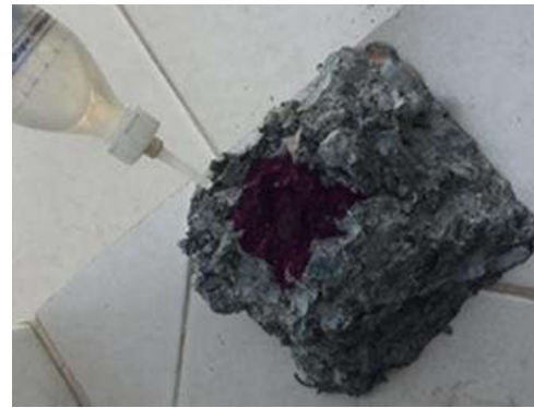
Fig. 12 Corrosion test-concrete with 2% Steel Scrap
