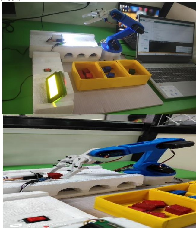
FIGURE 3.1 System Design with Colour Sensor
