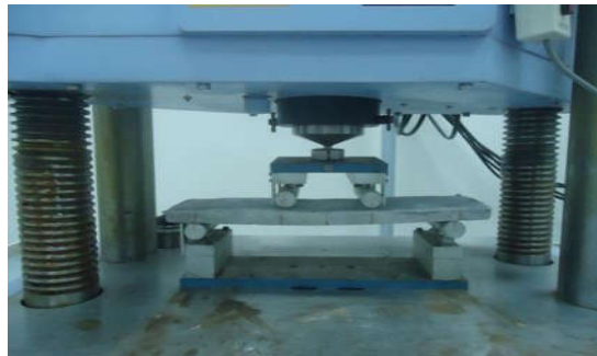
Figure 7 Ferro-cement Laminate under Flexure Test
