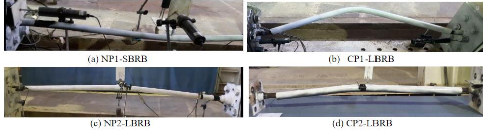
Fig.6. Overall buckling figures of specimens at the end of the test.
