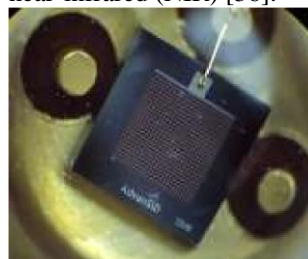
Figure 1. SiPM electronics schematic and a commercial SiPM (AdvanSiD, Trento, Italy).
