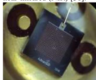
Figure 1. SiPM electronics schematic and a commercial SiPM (AdvanSiD, Trento, Italy).
