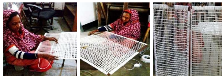
Figure 2: Preparation of polypropylene mesh and Nylon Mesh
